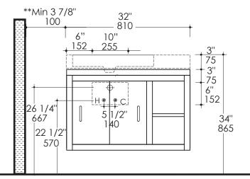
\*\* ADA floor clearance space required on the sink side due to off-centered faucet.
